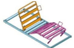
Articulated sleep deck with a head section fitted with a gas spring
